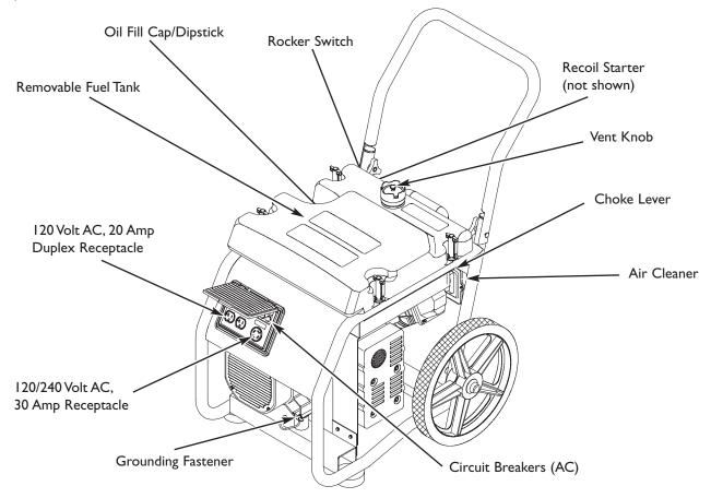
**I 20 Volt AC, 20 Amp, Duplex Receptacle** — May be used to supply electrical power for the operation of I 20 Volt AC, 20 Amp, single phase, 60 Hz electrical lighting, appliance, tool and motor loads.
